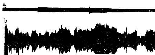
Fig. 4. Subharmonic component of cavitation noise recorded during irradiation of thalamus (a) and region including boundary separating heterogeneous structures (b). f = 1.98 MHz, I_F = 430 \text{ W} \cdot \text{cm}^{-2} , t = 5.0 sec.
